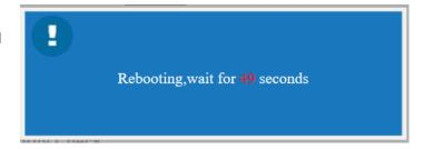
**Step 4** When the timer reaches zero you will be redirected to the login screen once more. The second and final part of the firmware upgrade is now complete. Log in to the CPE, confirm the correct firmware version is still showing in the About tile, and proceed with activation via existing process.
